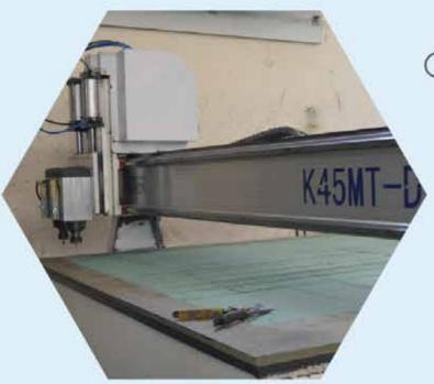
CNC ROUTER MACHINE BED SIZE 2MX4.5M
